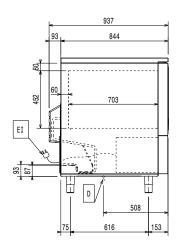
Drain Electrical inlet (power) ΕI Refrigerant Outlet
